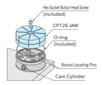
2-2. • Tighten the cam cylinder to clamp the locking ring. (Recommended Tightening Torque:15N·m) • After clamping the screw should be removed from the locking ring.
