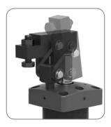
The 8700 series pneumatic lever clamp features an arm that arcs up and out of the way on a single plane. Since the arm does not rotate to the side like a swing clamp, it remains completely within the clamp's footprint while in the open position. This helps to eliminate interference with adjacent components on crowded fixtures.
